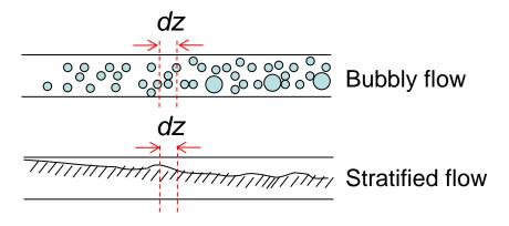
where  $\alpha_k$ : Volume fraction of k-phase, ( $\alpha_v + \alpha_l = 1$ )
